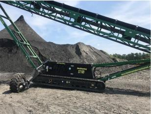
Designed for use in any terrain, the All-Terrain stackers, ranging from 60' to 150', are easily moved site to site without the need to remove the wheels for transport. Built-in levelling indicators allow operators to position the stacker regardless of the ground evenness, with independent hydraulic jack legs to stabilize once in place. The McCloskey design also eliminates the need for any additional equipment, delivering a clean radius without material buildup.
