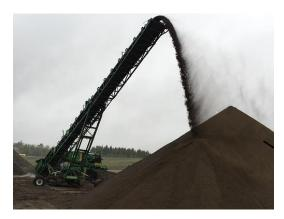
Designed for use in any terrain, the stackers, ranging from 60' to 150', are easily moved site to site without the need to remove the wheels for transport. Built-in levelling indicators allow operators to position the stacker regardless of the ground evenness, with independent hydraulic jack legs to stabilize once in place.
